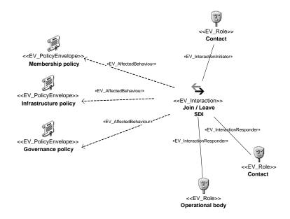
Figure 2.5: Join and Leave SDI interactions in UML (shown in one diagram, but they are two different interactions)
