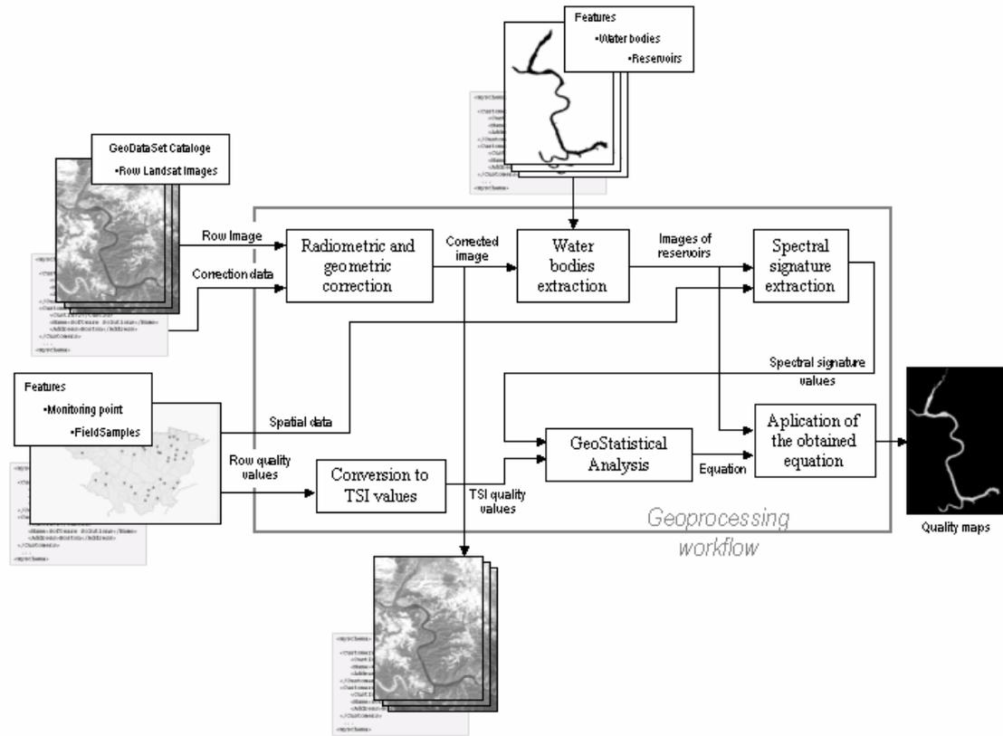
Figure 1: Geoprocessing Workflow applied in order to obtain the final quality maps.
