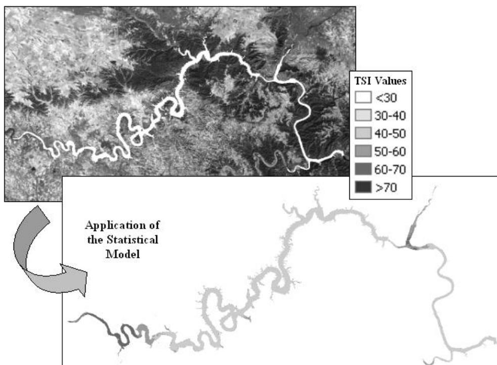
**Figure 2:** TSI maps for the Mequinenza reservoir and the Ribarroja reservoir calculated from Landsat TM reflectance through the obtained statistical model.
