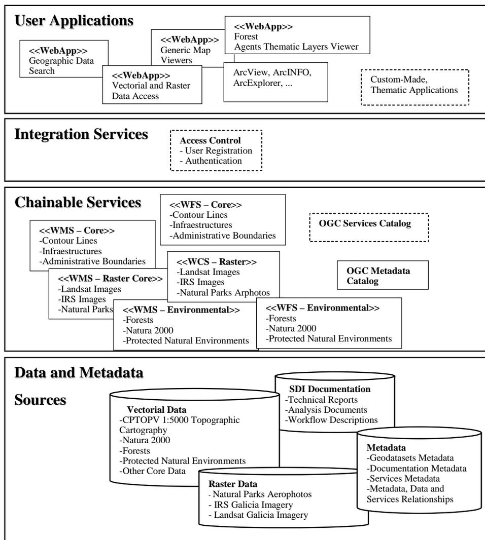
Fig. 1 Service-oriented view. Dotted lines show elements not yet finished or integrated
