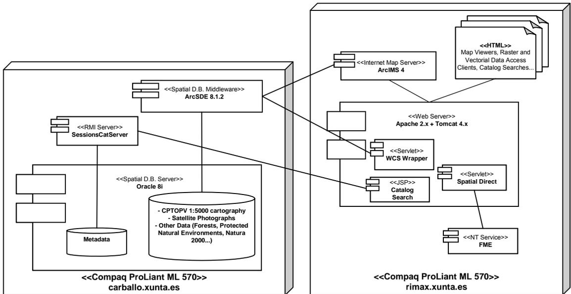
Fig. 2 Deployment diagram
