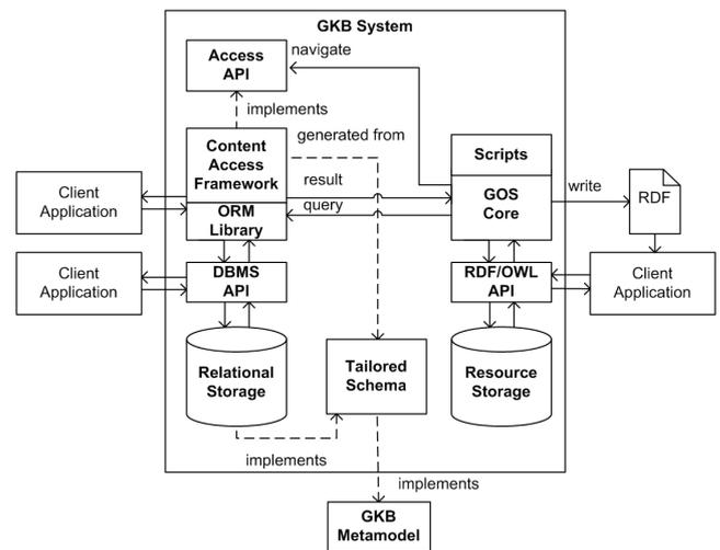
Figure 2: The architecture of the GKB System
