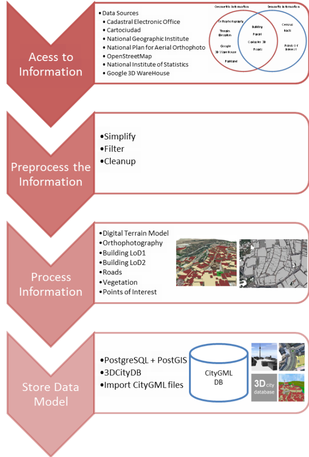
Figure 3: workflow for creating 3D city models from free data sources
